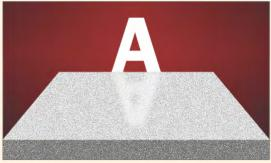
(A) Before TerrazzoShine: Mechanical deterioration, chemical attack, residue, and contamination caused by cleaning and polishing agents diffuse and absorb light, reducing the floor's reflective characteristics.
