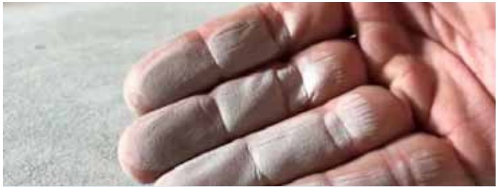
Excessive dusting of a concrete floor 2
