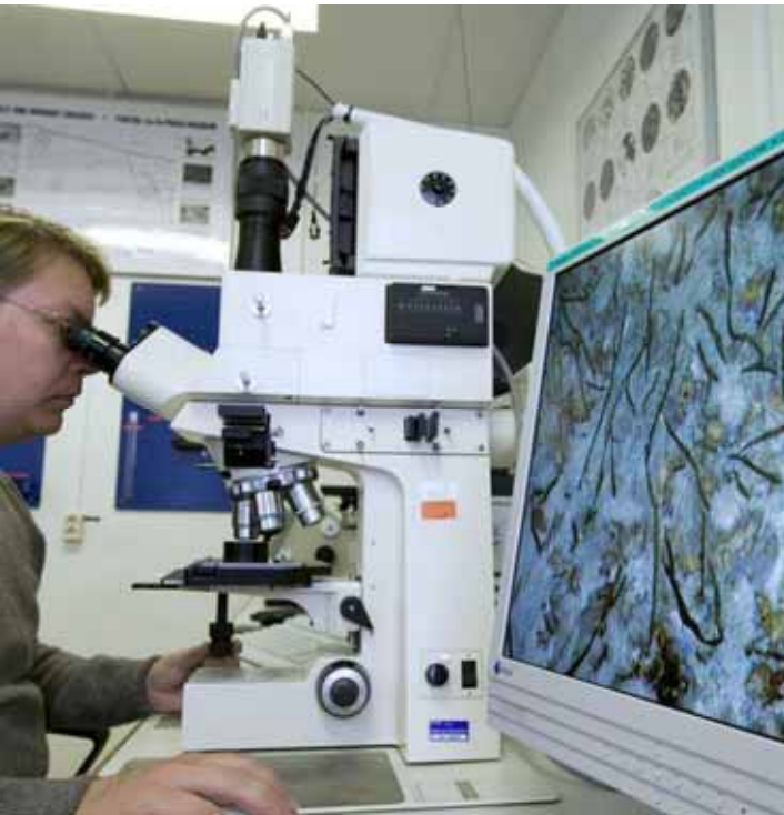
A researcher using thin section petrography for analysis 5
