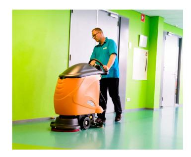
**Equipment:** Use mechanized cleanrer with a soft nylon bristle brush at the lowest speed.
